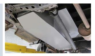
This replacement tank kit from Long Range Automotive of Melbourne, Australia was developed to meet the needs of North American pick up owners. The goal? To provide additional fuel capacity from a high-quality aluminized steel replacement tank that integrates seamlessly with factory fuel systems and emission controls in North American vehicles.
